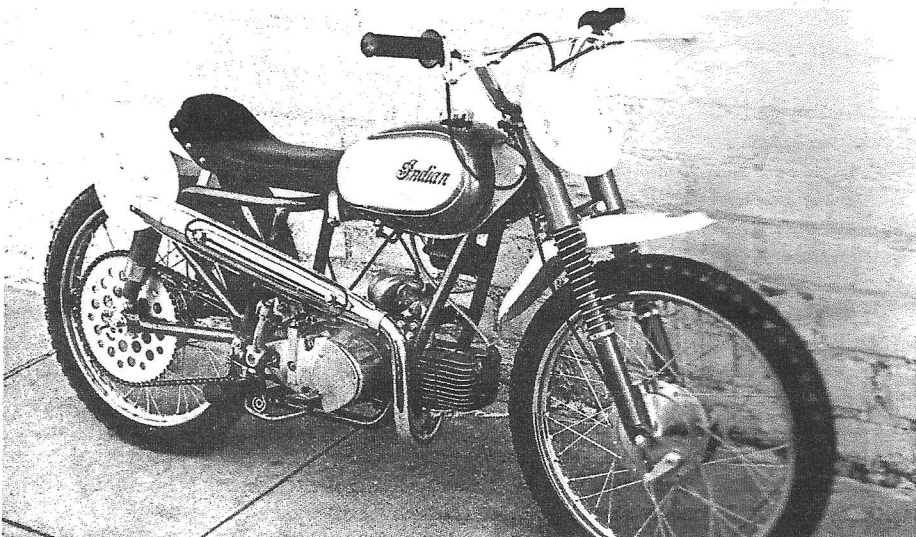
FINISHED in blue and white, this mini-motorcycle features a 40-inch wheelbase, 23-inch saddle height, two brakes, front and rear suspension.
