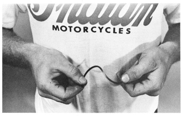
Indian now has a stock of 100 cc Fuji piston rings, made of a new, special flexible steel alloy. We have never before been able to offer rings of this quality. The new rings will fit all 8 H.P. pistons as well as the new 10 H.P. piston.
