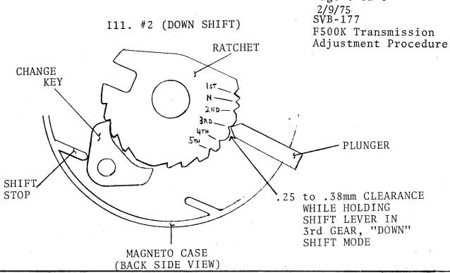
III. #3 ADJUSTMENT OF SHIFTER RATCHET MECHANISM
